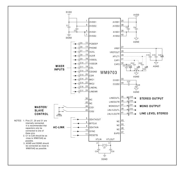
Figure 19 External Components Diagram
