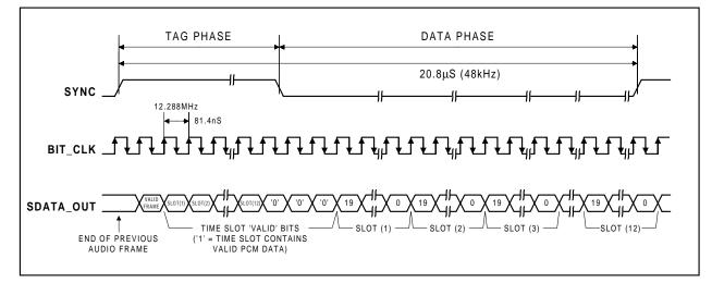
Figure 13 AC-link Audio Output Frame
