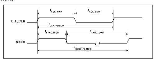
Figure 4 Clock Specifications (50pF External Load)
