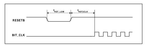
Figure 2 Cold Reset Timing
