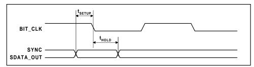
Figure 5 Data Setup and Hold (50pF External Load)
