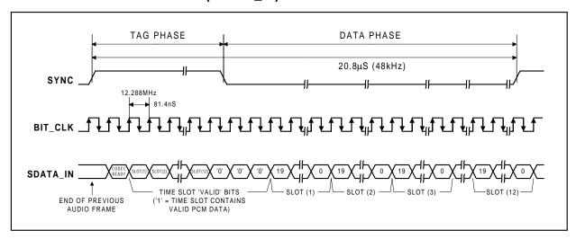
Figure 11 AC-link Audio Input Frame
