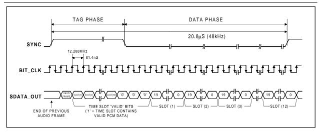
Figure 9 AC-link Audio Output Frame
