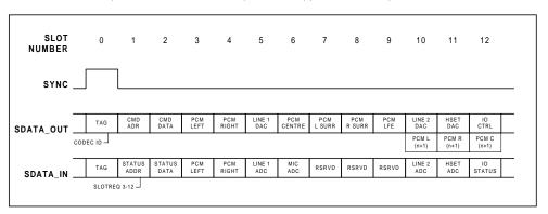
Figure 8 AC'97 Standard Bi-directional Audio Frame
