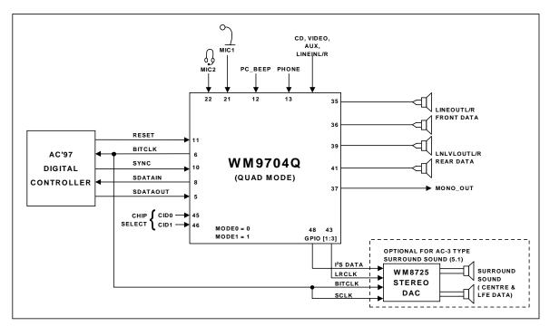
Figure 7 WM9704Q in Typical Quad Mode Application
