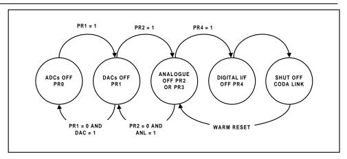
Figure 14 The WM9704Q Powerdown/Flow with Analogue Still Alive
