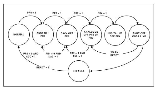
Figure 13 An Example of the WM9704Q Powerdown/Powerup Flow
