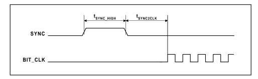
Figure 3 Warm Reset Timing
