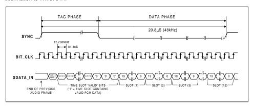
Figure 10 AC-link Audio Input Frame
