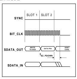
Figure 1 AC-Link Power down Timing
