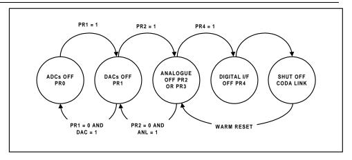
Figure 13 WM9701A Power Down/Flow with Analogue Still Alive
