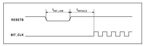
Figure 2 Cold Reset Timing
