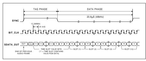
Figure 8 AC-link Audio Output Frame
