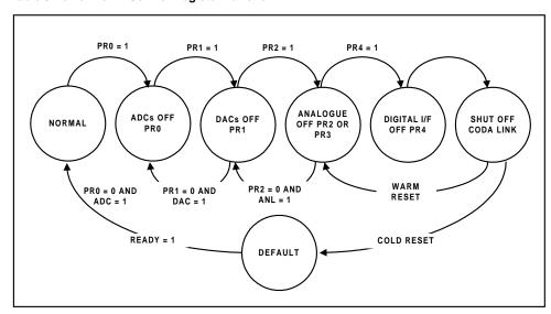
Figure 12 An Example of WM9701A Power Down/Power up Flow
