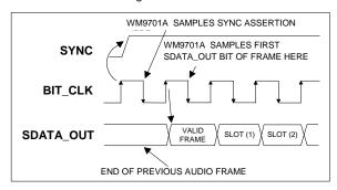
Figure 9 Start of an Audio Output Frame
