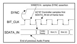
Figure 11 Start of an Audio Input Frame
