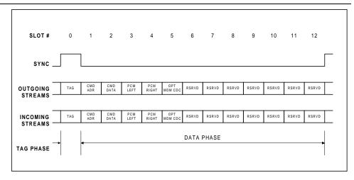
Figure 7 AC'97 Standard Bi-directional Audio Frame
