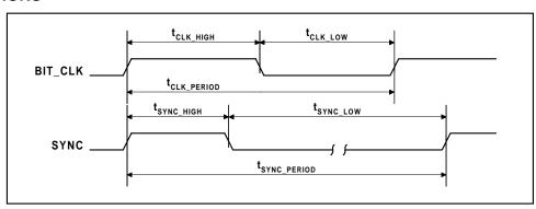
Figure 4 Clock Specifications (50pF External Load)
