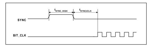
Figure 3 Warm Reset Timing
