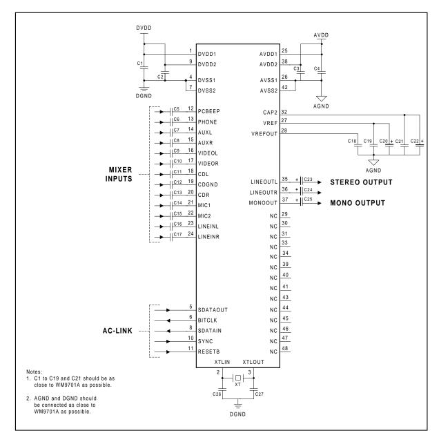
**Figure 14 External Components Diagram**
