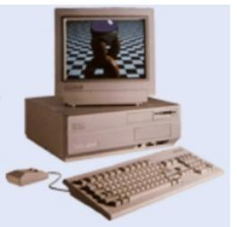
Amiga 2000B - Designed in the USA and basically a machine inbetween 2000A and a cost reduced version of Amiga 500. Thanks to the cheaper and more logical design, 1Mb RAM moved onto the motherboard. Known as B2000 in the UK.
