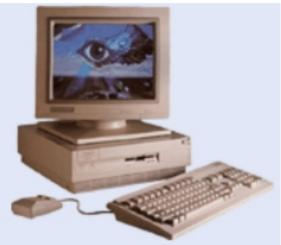
It was sold with two operating systems, Workbench 2.04 and the Unix System (SVR4) V. It also came with networking capabilities such as TCP/IP.
