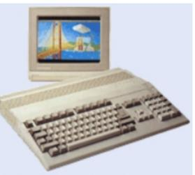
The most common way to upgrade was 512Mb extra RAM (including a battery-backed clock) which fitted at the bottom of the case. An extra floppy disk drive was common as well. Additionally, a hard disk and up to 8Mb RAM could be plugged into the DMA expansion slot on the left side.
