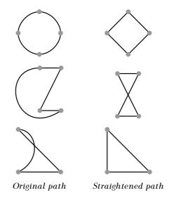
**Figure11**: The operation of straightening of a path typically does not change the orientation of a path (top); in general, however, this may happen—middle and bottom pictures show how a non-zero turning number can be changed to zero and vice versa. The latter situations, fortunately, are rather unlikely in fonts.
